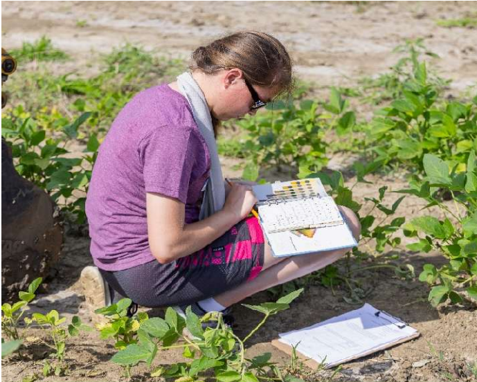
Biene determines Munsell soil color at the soil pit
